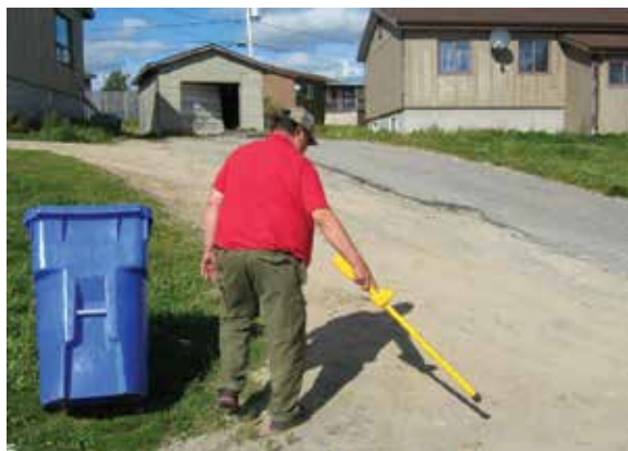
Field mapping and teamwork locating infrastructure assets using a handheld GPS device, metal detector, heavy machinery and other equipment in collaboration with Ouje-Bougoumou staff.
